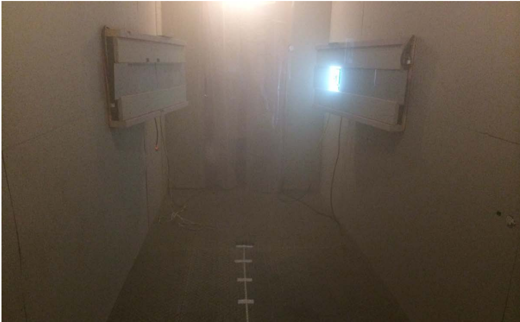
Figure 8. Mounting brackets for test signs (shown without ambient smoke).
